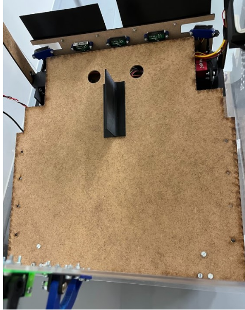
Figure 3.14: 15° plate with middle rib, and the thin flexible sheets on the front
